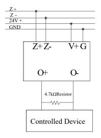
Note: The controlled device should be polarized, high resistance in reversed direction.
