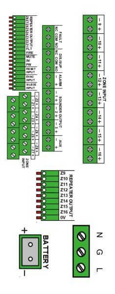
FAULT (NC, COM, NO): Fault output terminal.
