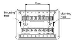
J11, J12: Output terminal of gas extinguishing Start command, connect with cylinder solenoid.
